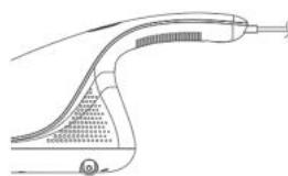
3. Holding the handle, slightly force the front two sensor wheels to press down, trigger the micro switch, the UV lamp is turned on, the machine enters the vacuum, the vibration tapping, the hot air drying and the ultraviolet lamp sterilization state.
