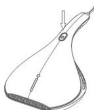
2. Press the key to open, the main vacuum motor and the beat motor start, the machine then enters the state of vacuuming and vibrating. The hot air will blow outside through the hot air outlet at the bottom. The machine will then turn on the hot air drying function.
